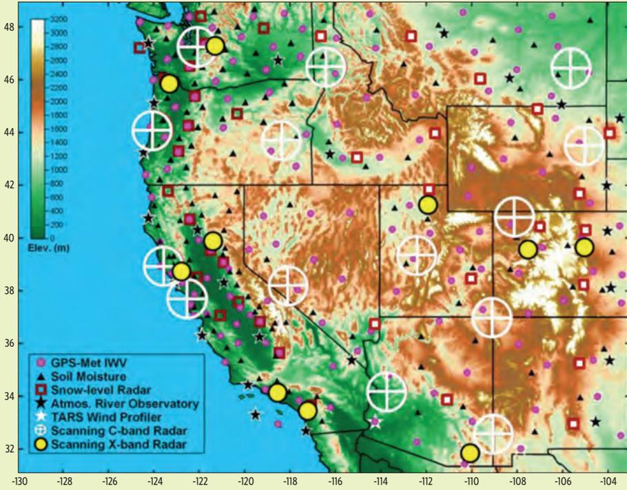
**Schematic network of new land-based sensors** to improve monitoring, prediction and climate trend detection for hydrometeorological conditions that create extreme precipitation and flooding. Offshore coastal sensors not shown.
