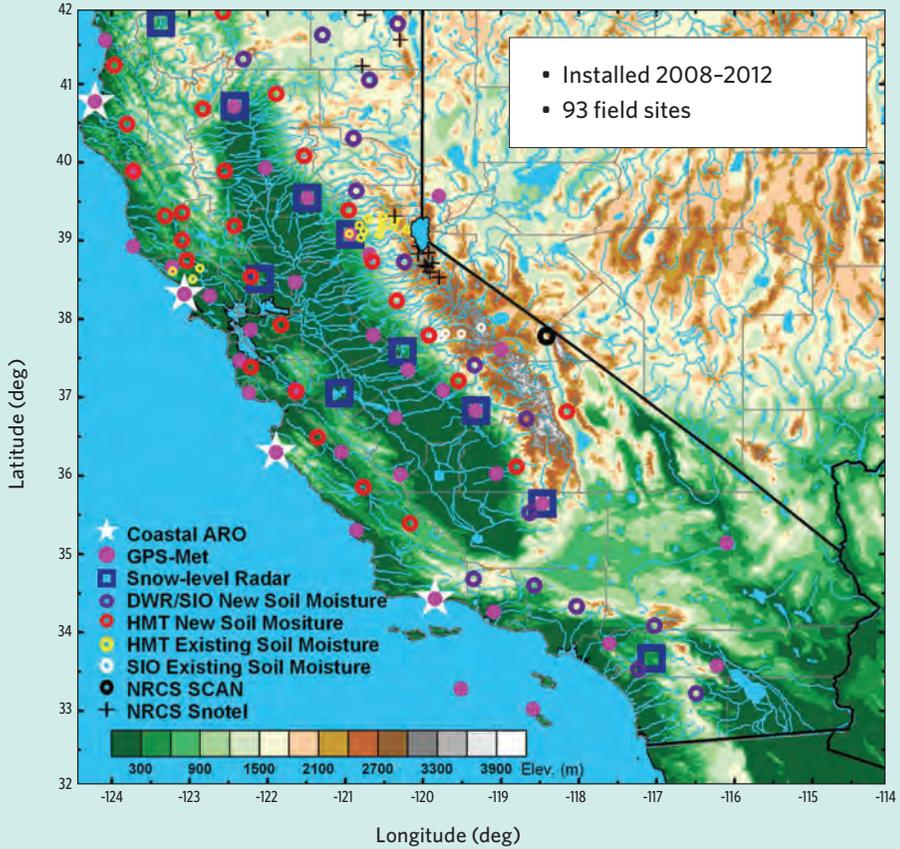
**An AR-focused long-term observing network** is being installed in California as part of a 5-year project between CDWR, NOAA and Scripps Inst. of Oceanography.
